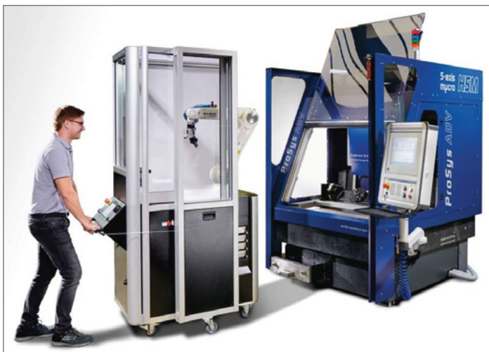
Mobile MRC Flextray Cell docking to machine
