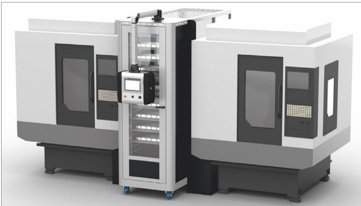
MRC flextower with 2 CNC machines
