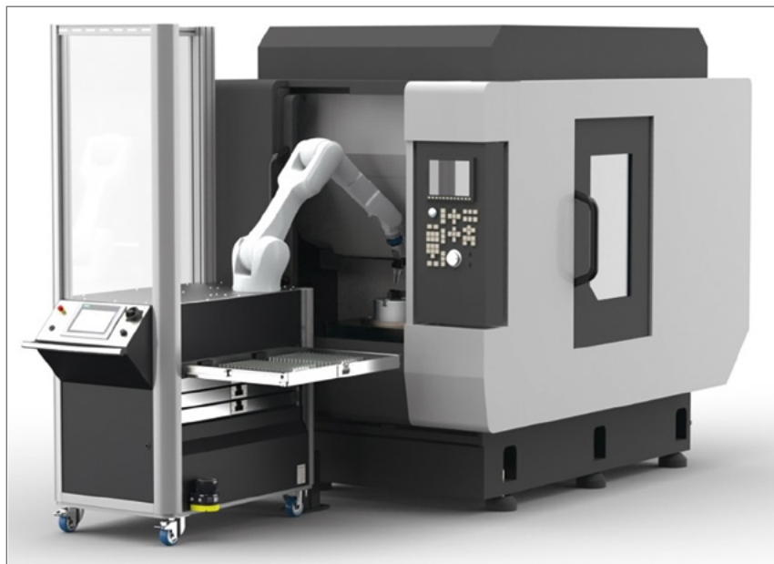
CNC milling center connected to machine front
