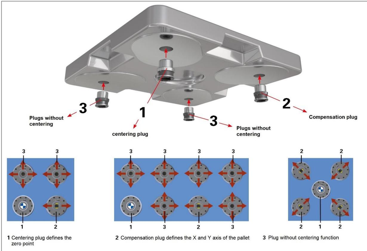
Figure 4 – Recommended clamping plug arrangements
