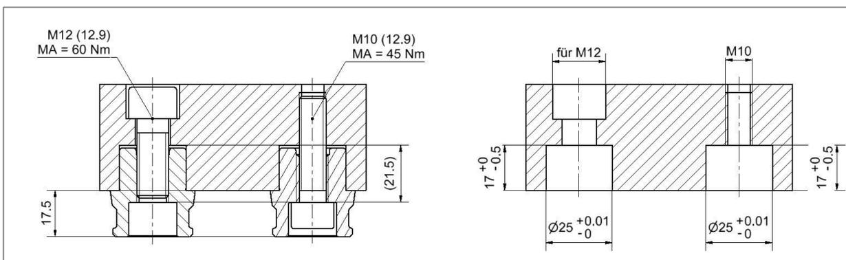
Figure 2 – Clamping plug holes
