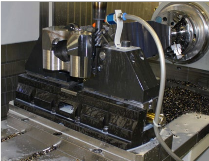
BSM-500 as a steady rest. The workpiece is clamped with a 3-jaw chuck, the centric vise is used purely for clamping support.
