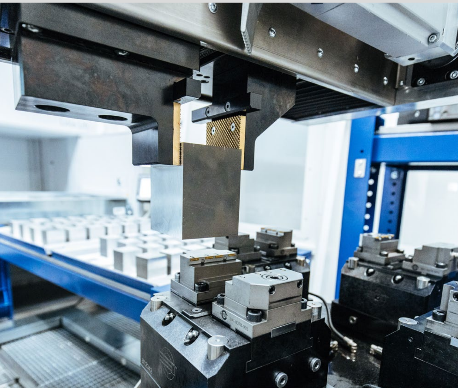
VBA Profi Line centric vise with OP10 pendulum Mastergrip jaws and workpiece contact control
