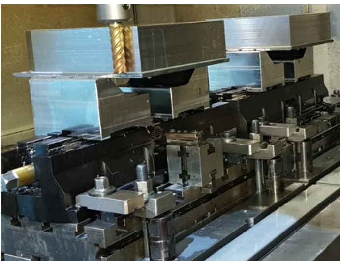
2 BSM-500 vises in series. Clamping is achieved with Mastergrip jaws that can be rotated for clamping smaller workpieces.
