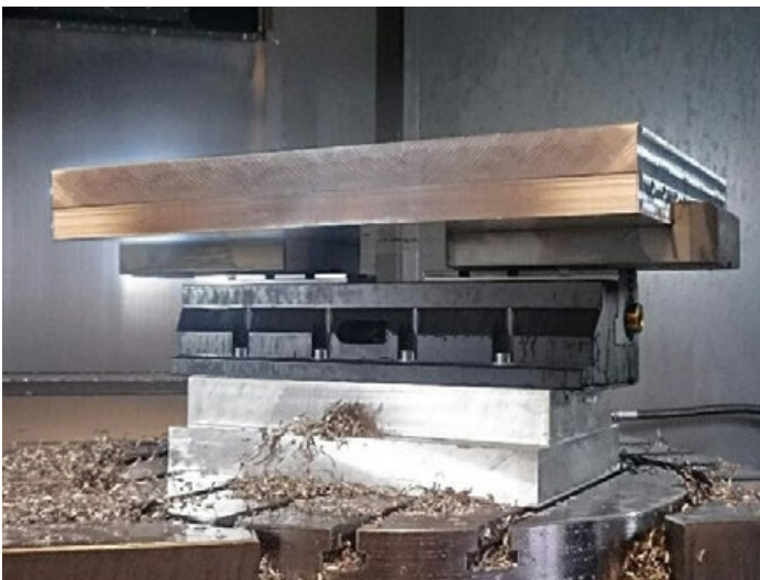
BSM-500 with protruding jaws for clamping workpieces up to 636 mm. The vise is mounted on a riser for optimum accessibility during 5-axis machining.
