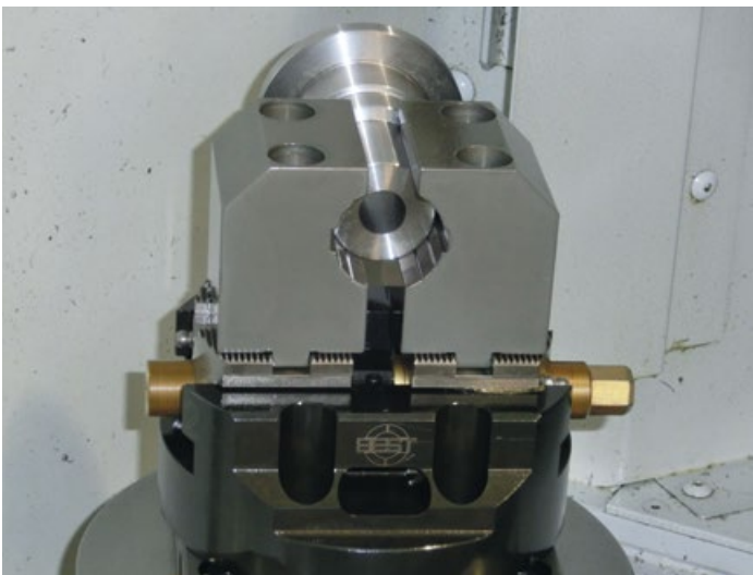
BSM-140 with form jaws (customized) for clamping a turned part with a 35 mm diameter.
