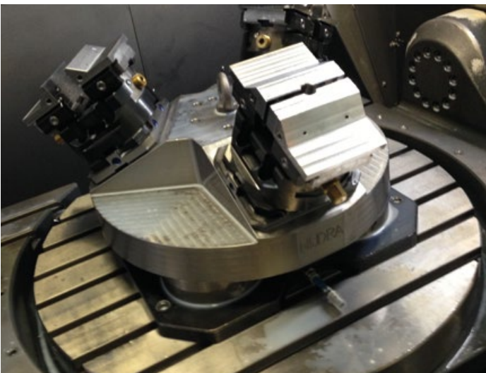
3 BSM-140 vises with form jaws on a 5-axis pyramid. The vises are each mounted on a mechanical zero-point plate. The pyramid is picked up on a pneumatically actuated zero-point clamping system.
