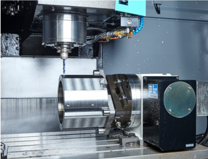
BSM-250 on Kitagawa rotary table. Clamping set-up with Vario jaws for reworking of a housing.
