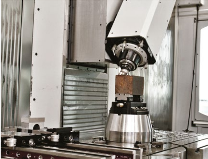
BSM-250 on a 5-axis riser for optimum accessibility during 5-axis machining.
