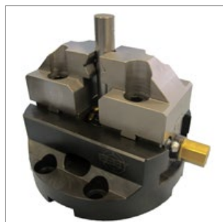
Special prismatic jaw 301-0020-001 for BSM-115-KV, clamping range 6-20 mm horizontal and vertical
